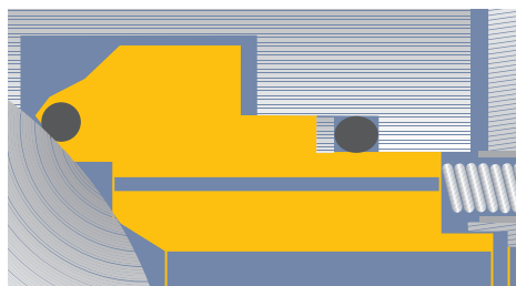
Sealing system: PMSS, primary metallic/ secondary soft-seated
