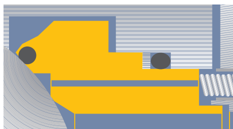
sealing system: PMSS, primary metallic / secondary soft-seated
